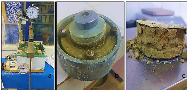
Figure 6. Oedometric frames with modified cell support and resistance (LNHC-Batna).
